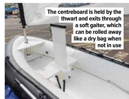
The centreboard is held by the thwart and exits through a soft gaiter, which can be rolled away like a dry bag when not in use
