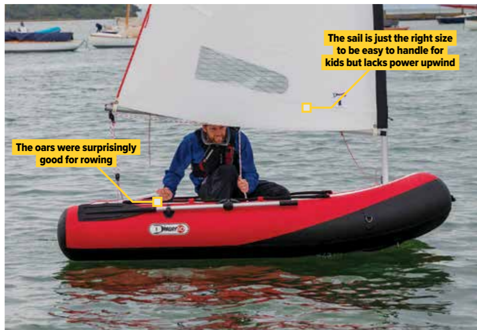
The sail is probably a touch far forward relative to the daggerboard, giving lee helm
