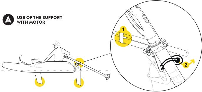
For optimal use of your Tiwal as a motorized tender, it is recommended to sail with the daggerboard and rudder lowered (be careful, however, to raise these two elements when arriving at the beach).
