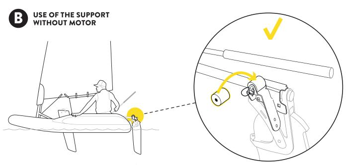
Use the roller in the motor cradle to prevent the stick from colliding with it.
